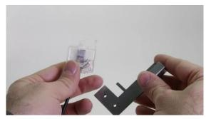
Select a location on the machine to mount the receiver so that the TriTeq electronic key can properly communicate with the lock. The location will vary depending on your machine. You should select the same mounting location on all your vendors to avoid confusing the route drivers and service personnel.
