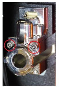
Fasten the latch module to the housing using two #5 set screws and the 2.5 mm allen driver.
