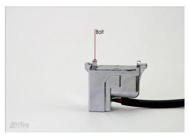
Incorrect Position: This view the bolt is extended. Do not attempt to mount the latch module if the bolt is extended above the surface of the front flange as shown. Do not attempt to push or force the bolt down below the surface of the front flange to the retracted position.
