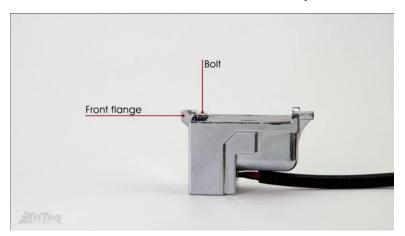
Correct Position: This view shows the retracted position of the bolt – flat with or below the surface of the front flange. The bolt should be in this position when you receive this lock kit from TriTeq. If the latch module is as shown, proceed to step 4.
